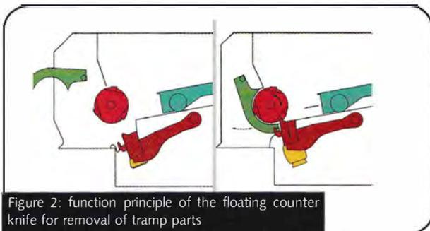
Figure 2: function principle of the floating counter knife for removal of tramp parts
